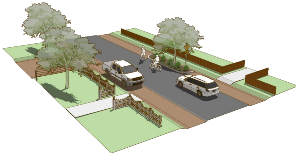
Figure 34. This concept from the STAR Guide shows some potential features of a yield roadway. People walking, bicycling, and driving mix in the road. What the yield roadway design adds are features and characteristics that serve to keep car traffic at slower speeds. The actual travelway width is narrowed from the typical 20 ft., with no yellow centerline, and the roadside can have gravel or dirt shoulders that serve as parking lanes, places to pull aside to yield to an oncoming car, or islands that can have plants, stormwater management, signs, or other features.
