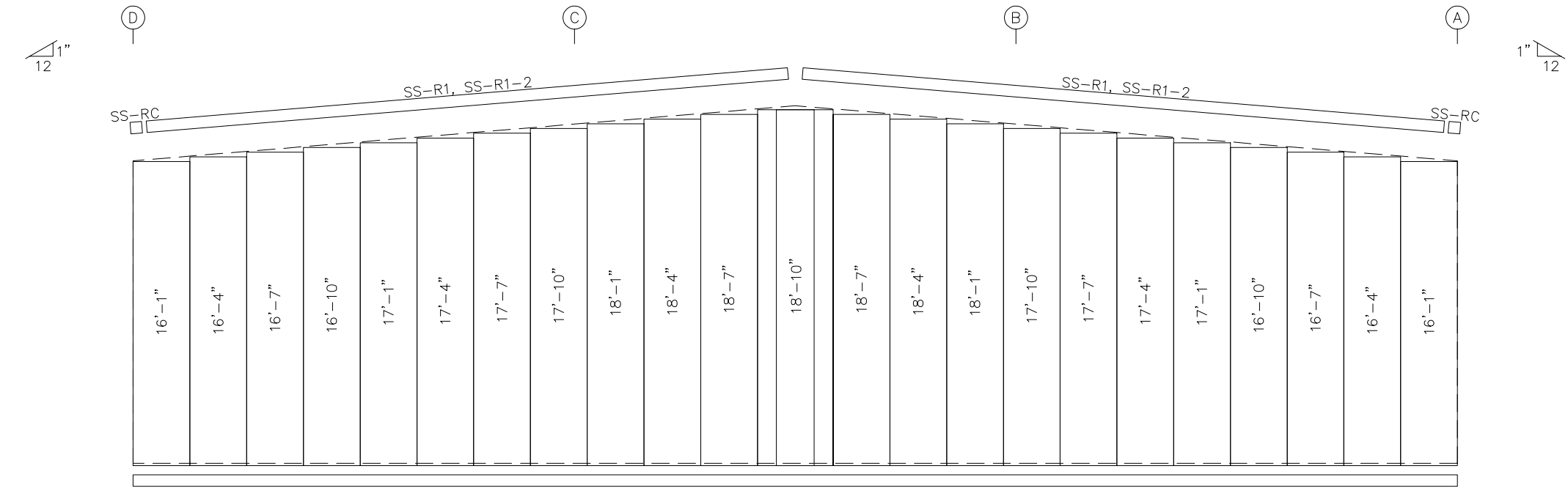
ENDWALL SHEETING & TRIM: FRAME LINE 1
