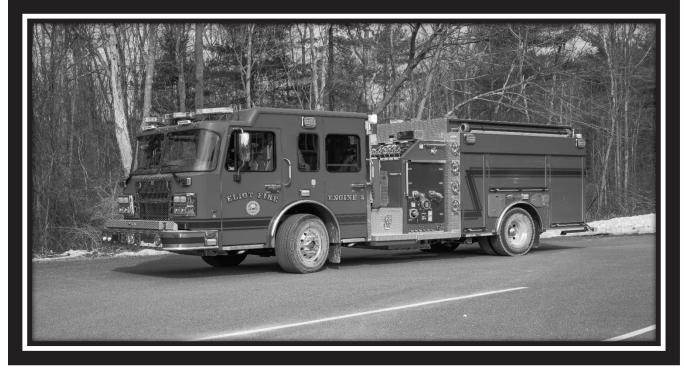
Old Fire Department Pumper Truck – 1996 Central States, this truck also held a 1000 gallons of water and pumped 1250 gallons per minute. This truck served the Town of Eliot, for 26 years and was traded in for the new truck.
